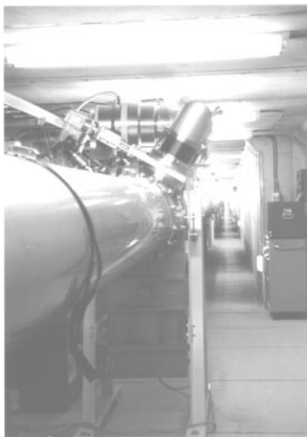
Figure P3.6 The 300-m Fabry–perot cavity of the TAMA gravitational wave detector. (Courtesy of A. Araya et al. [40].)
